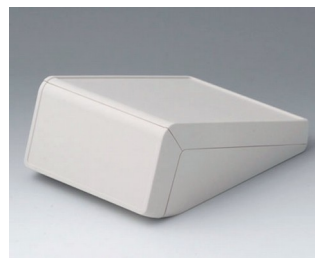
B4056137 UNITEC M, 0.6/1.4 ABS (UL 94 HB) off-white RAL 9002 148x210x80mm IP 40
