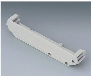
B6724333 RAILTEC SUP. 72, end section PA 6 (30) (UL 94 V-0) light grey 82x11,2x16mm
