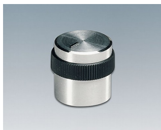
A1416469 TUNING KNOB, with lateral screw fixing ABS (UL 94 HB) brilliant 15,9x15,2mm 6mm
