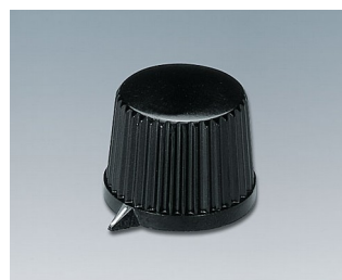
A1313540 TUNING KNOB, with lateral screw fixing PF (UL 94 V-0) black RAL 9005 20x15,4mm 4mm
