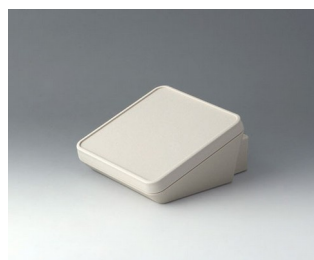
B4414307 PROTEC 140, Vers. III ASA+PC (UL 94 V-0) off-white RAL 9002 140x160x76mm IP 65 opt.
