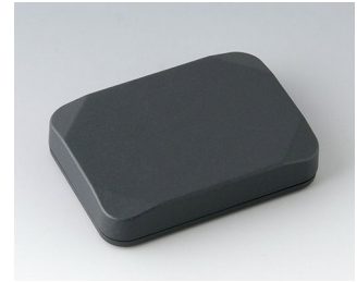
B1824118 MINI-DATA-BOX E50, flat ASA+PC (UL 94 V-0) anthracite grey RAL 7016 70x50x15mm IP 65 opt., IP 40
