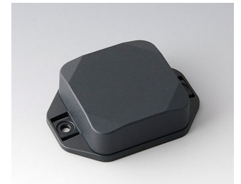
B1804228 MINI-DATA-BOX SF50, high, with flanges ASA+PC (UL 94 V-0) anthracite grey RAL 7016 50x50x20mm IP 65 opt., IP 40
