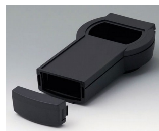
A9078209 DATEC-CONTROL M, Vers. II ABS (UL 94 HB) black RAL 9005 243x130x60mm IP 54 opt.
