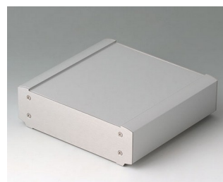
B3407013 SMART-TERMINAL 160 Aluminium AlMgSi 0,5 matt anodised 164x170x50mm
