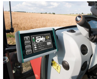
ISOBUS terminal for tractors and self-propelled machines
