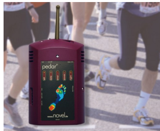
Dynamic pressure measuring between foot and shoe
