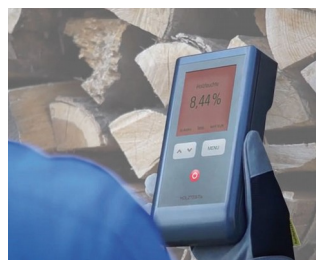
Wood moisture measuring device
