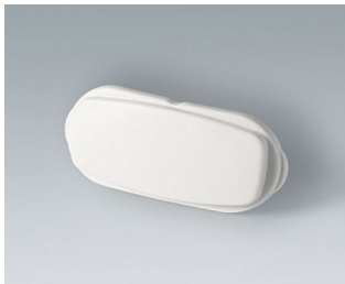
B2811207 End part ASA+PC (UL 94 V-0) off-white RAL 9002
