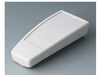
A9067117 SMART-CASE L, Vers. II ABS (UL 94 HB) off-white RAL 9002 140x62,7x30,5mm IP 65 opt., IP 40
