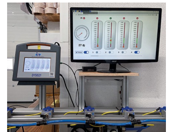
Monitoring system for cleaning nozzles
