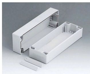
C2108242 ROBUST-BOX WIDTH 80, Vers. II PC (UL 94 HB) light grey RAL 7035 240x80x80mm IP 66
