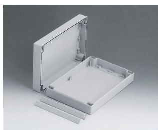
C2016241 ROBUST-BOX WIDTH 160, Vers. I ABS (UL 94 HB) light grey RAL 7035 240x160x60mm IP 66
