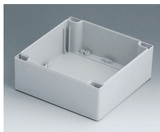
C2161602 Case shell 160, with tongue PC (UL 94 HB) light grey RAL 7035 160x160x60mm
