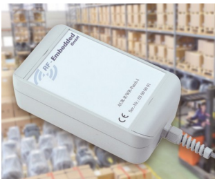
Active UHF RFID system
