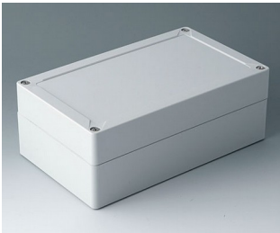
C7020041 IN-BOX ABS (UL 94 HB) light grey RAL 7035 202x122x75mm IP 66, IP 67, IK 07
