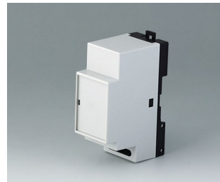
B6511111 RAILTEC B, 2 modules, Vers. XI PC (UL 94 V-0) light grey RAL 7035 35x86x58mm
