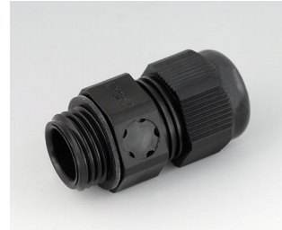
C2316919 Cable gland M16x1.5, pressure compensation PA black RAL 9005
