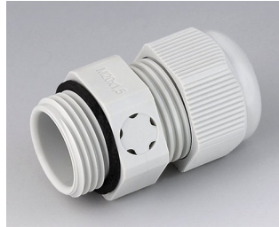
C2320917 Cable gland M20x1.5, pressure compensation PA light grey RAL 7035 IP 68
