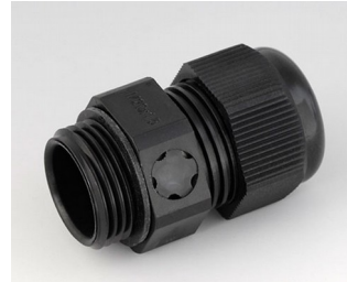
C2320919 Cable gland M20x1.5, pressure compensation PA black RAL 9005 IP 68
