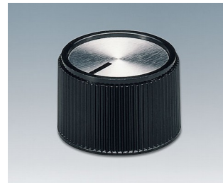
A1324260 TUNING KNOB, with lateral screw fixing PF (UL 94 V-0) black/alu 24,3x16mm 6mm
