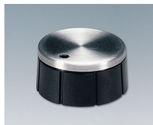
A1624260 TUNING KNOB, with lateral screw fixing ABS (UL 94 HB) black/alu 24x12,4mm 6mm
