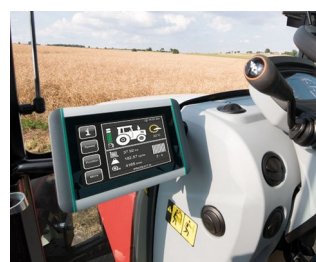
ISOBUS terminal for tractors and self-propelled machines
