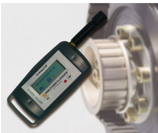
Tension meter for measuring belt pretension
