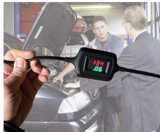
Voltage and current display during trickle charging
