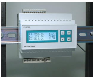
Power measuring device for energy analysis
