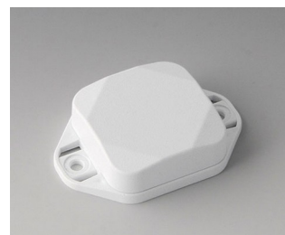
B1802127 MINI-DATA-BOX SF40, flat, with flanges ASA+PC (UL 94 V-0) traffic white RAL 9016 40x40x15mm IP 65 opt., IP 40
