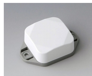
B1802226 MINI-DATA-BOX SF40, high, with flanges ASA+PC (UL 94 V-0) traffic white RAL 9016 40x40x20mm IP 65 opt., IP 40
