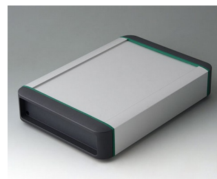
B3407021 SMART-TERMINAL 200 Aluminium AlMgSi 0.5 matt anodised 242x170x50mm IP 54
