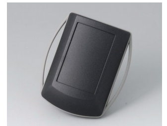
B7040229 ERGO-CASE XS ABS (UL 94 HB) black RAL 9005 82x56x24mm IP 42
