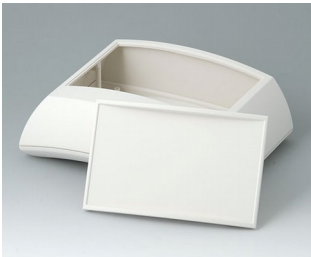
B7025237 ERGO-CASE L, high ABS (UL 94 HB) off-white RAL 9002 150x200x69mm IP 40
