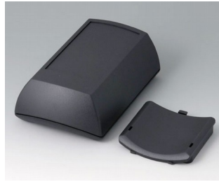
B7015109 ERGO-CASE M, high ABS (UL 94 HB) black RAL 9005 150x100x55mm IP 54 opt.
