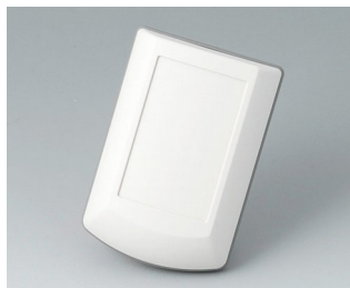
B7040237 ERGO-CASE XS ABS (UL 94 HB) off-white RAL 9002 82x56x24mm IP 42
