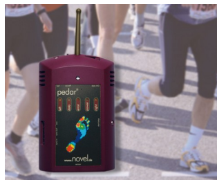
Dynamic pressure measuring between foot and shoe
