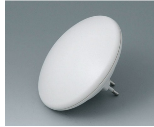
B5011127 ART-CASE R110 H PC+ABS (UL 94 V-0) off-white RAL 9002 ø110x38mm IP 40
