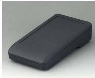
A9006108 DATEC-COMPACT M ASA+PC (UL 94 V-0) lava 172x92x39mm IP 65
