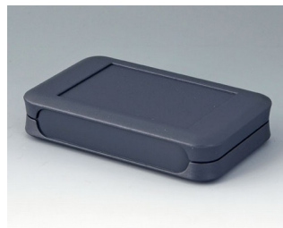
A9052108 SOFT-CASE L ABS (UL 94 HB) lava 73x117x24mm IP 54 opt., IP 40
