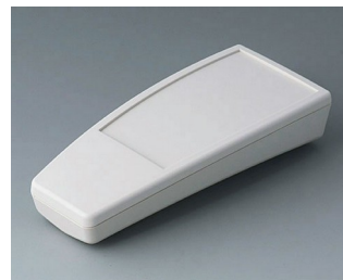
A9068117 SMART-CASE XL, Vers. II ABS (UL 94 HB) off-white RAL 9002 168x74.4x35.4mm IP 65 opt., IP 40
