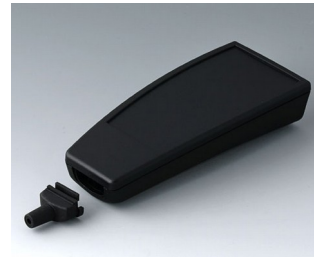
A9067339 SMART-CASE L, Vers. IV ABS (UL 94 HB) black RAL 9005 140x62.7x30.5mm IP 65 opt., IP 40
