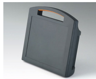
B4213208 CARRYTEC L ASA+PC (UL 94 V-0) lava 348x303x117mm IP 54 opt.
