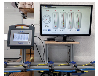
Monitoring system for cleaning nozzles
