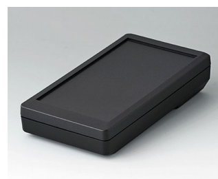
A9073119 DATEC-MOBIL-BOX S, Vers. I ABS (UL 94 HB) black RAL 9005 152x83x33.5mm IP 65 opt.
