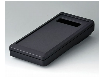
A9075219 DATEC-MOBIL-BOX L, Vers. II ABS (UL 94 HB) black RAL 9005 252x121x50mm IP 65 opt.
