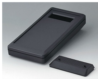
A9075209 DATEC-MOBIL-BOX L, Vers. II ABS (UL 94 HB) black RAL 9005 252x121x50mm IP 65 opt.
