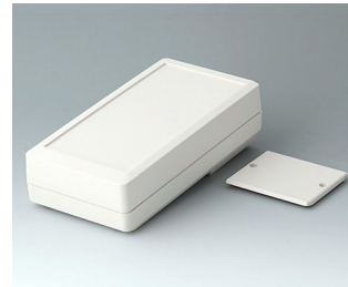
A9074127 DATEC-MOBIL-BOX M, Vers. I, high ABS (UL 94 HB) off-white RAL 9002 195x101x59mm IP 65 opt.
