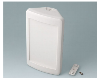
B4610207 SMART-CONTROL M, Vers. II ASA+PC (UL 94 V-0) off-white RAL 9002 173x101x59mm IP 55 opt., IP 40
