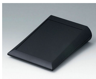
A0615009 COMTEC 150 F, Vers. I ABS (UL 94 HB) black RAL 9005 150x200x51.5mm IP 40
