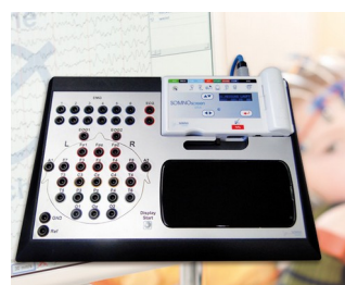
Stationary system for long-term EEG recordings
