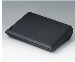
A0629109 COMTEC 290 H, Vers. I ABS (UL 94 HB) black RAL 9005 290x200x75.5mm IP 40
