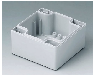
C1080802 Case shell 80, with tongue PC (UL 94 HB) light grey RAL 7035 80x80x40mm
