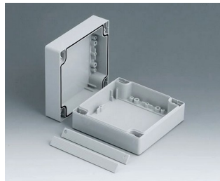
C201212 ROBUST-BOX WIDTH 120, Vers. II PC (UL 94 HB) light grey RAL 7035 120x120x60mm IP 66
