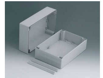
C2416242 ROBUST-BOX WIDTH 160, Vers. II PC (UL 94 HB) light grey RAL 7035 240x160x120mm IP 66
