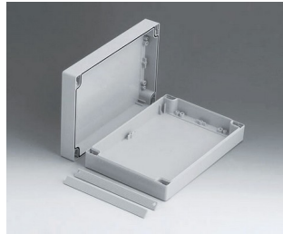
C2016242 ROBUST-BOX WIDTH 160, Vers. II PC (UL 94 HB) light grey RAL 7035 240x160x60mm IP 66
