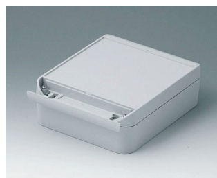
C6015181 SMART-BOX WIDTH 150 ASA+PC (UL 94 V-0) light grey RAL 7035 180x150x60mm IP 66
