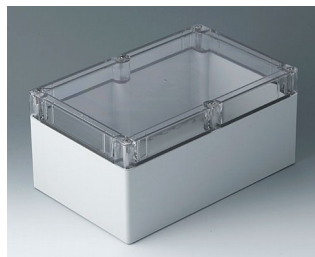
C7025095 IN-BOX PC light grey RAL 7035 252x162x120mm IP 66, IP 67, IK 08
