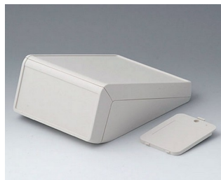
B4056217 UNITEC M, 1.4/1.4 ABS (UL 94 HB) off-white RAL 9002 148x210x80mm IP 40
