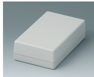
A9408341 SHELL-TYPE CASES G 155, Vers. I ABS (UL 94 HB) off-white RAL 9002 95x158x45mm IP 65 opt.
