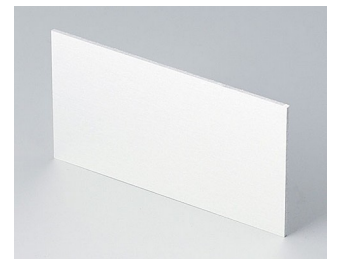
B6132112 Rear panel Aluminium matt anodised 73.5x39.6x1mm
