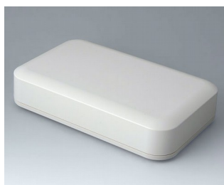
A9481107 EVOTEC 250, Vers. I ASA+PC (UL 94 V-0) off-white RAL 9002 250x155x54mm IP 65 opt., IP 40
