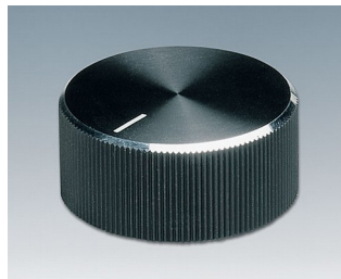
A1422260 TUNING KNOB, with lateral screw fixing ABS (UL 94 HB) black/alu 22.8x13mm 6mm
