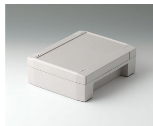
C8014182 SOLID-BOX 145 PC+ABS (UL 94 V-0) light grey RAL 7035 180x145x60mm IP 66, IP 67, IK 08
