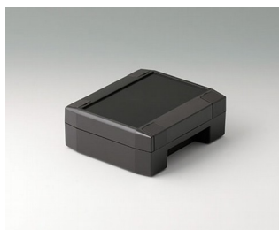
C8011131 SOLID-BOX 115 PC+ABS (UL 94 V-0) anthracite grey RAL 7016 135x115x50mm IP 66, IP 67, IK 08
